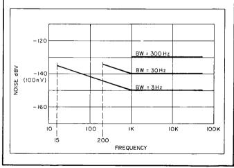
Noise Sidebands: > 70 dB below CW signal 10 Bandwidths away from signal.
